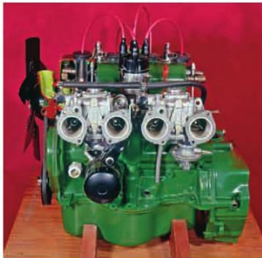
Standard 4-cylinder R8 Gordini engine. (©R)
