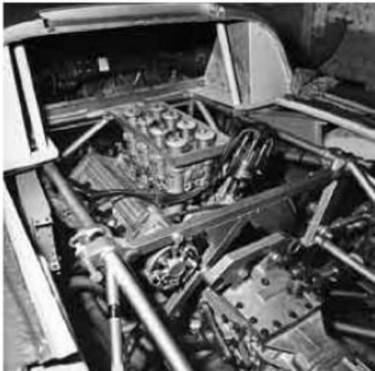
A tight squeeze: the V8 in the A211. (Photo AAA)
