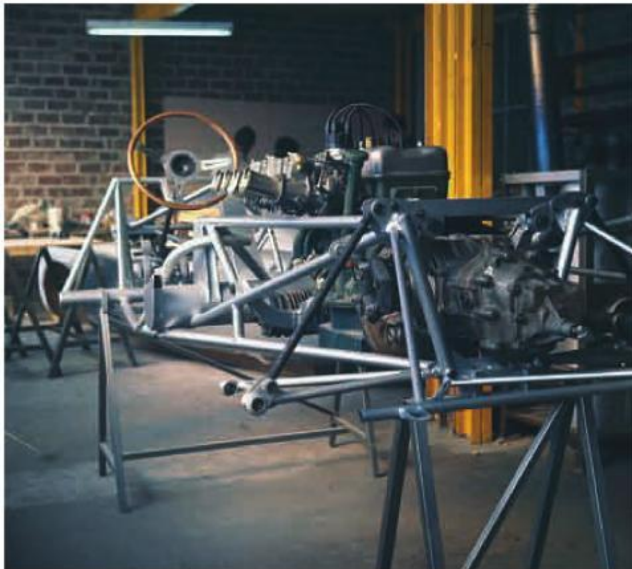
Twin overhead cam engine installed in the M63 chassis. (Photo CD)
